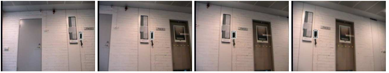
Fig. 9. Tracking of a landmark after 1, 10, 15, 20 frames with \delta = 5.0 and additional position prediction.
