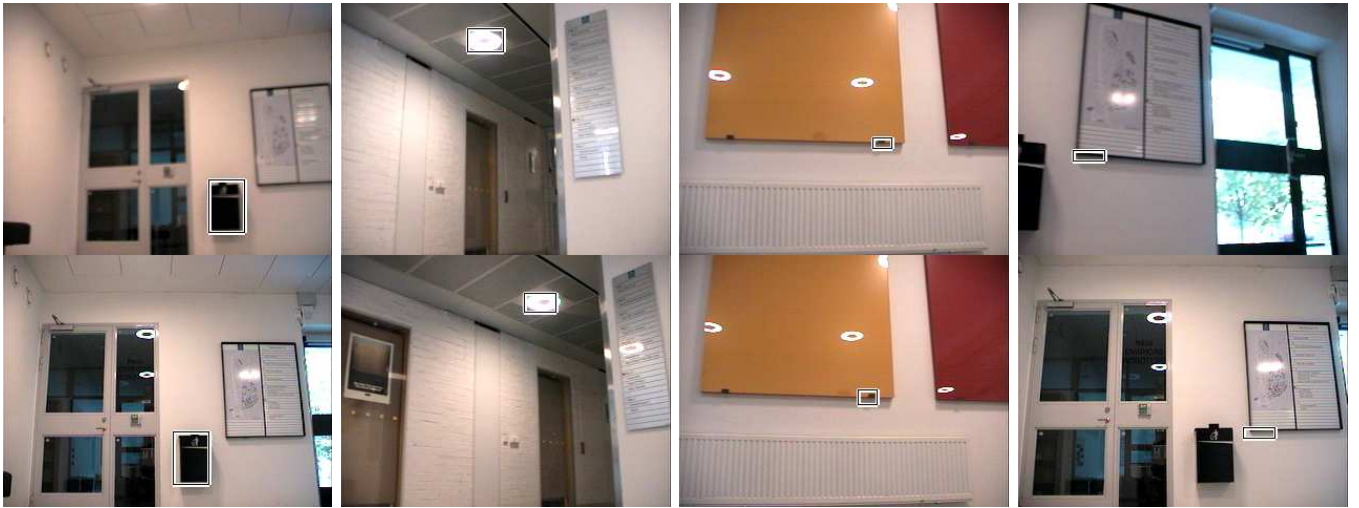
Fig. 10. Correct matches in loop closing situations: the first row shows a ROI in a current frame, the second row shows a previously stored ROI the current ROI was matched with. This situation usually occurred after the robot drove a circle and revisited the same area again.
