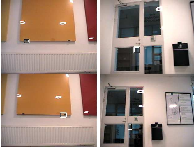
Fig. 11. False matches in loop closing situations: the first row shows a ROI in a current frame, the second row shows a previously stored ROI the current ROI was matched with. The matched regions are associated wrongly since they are highly ambiguous.
