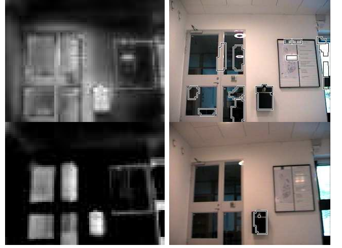
Fig. 4. Saliency maps (top, left: S_{bu} , bottom, left: S_{td} ) and MSRs in a loop closing example: Top: scene at beginning of sequence. Bottom: revisited scene, 592 frames later, searching for the black waste bin with top-down attention.
